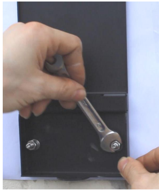
6.Tighten the screw with a wrench
