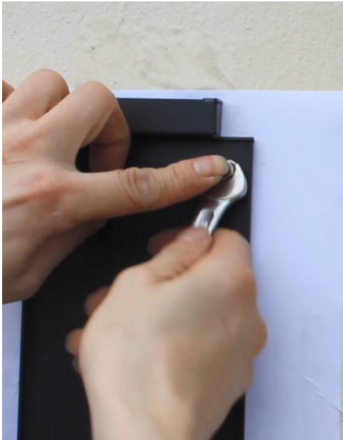
5.Tighten the screw with a wrench
